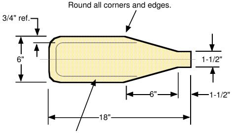
Apply 1-1/2" wide glass cloth tape to outside edges per sketch above. Use the T&G method of application.
